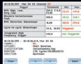
To further speed analysis, Gossen Metrawatt has added AnswerModules®, intelligent algorithms that help pinpoint the source and cause of power quality problems, to the MAVOWATT 40. These diagnostic and reporting tools are based on decades of analytical experience and bench-marking/troubleshooting work, as they convert raw data into precise answers for rapid decision-making.
